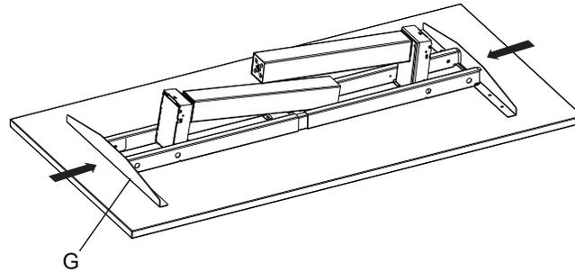
Install the cross brackets to the main frame
