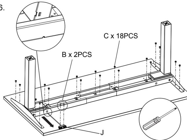
Ensure cable for controller passes through groove under table top before screwing onto table top
