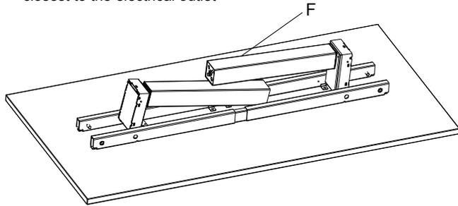
Put the main frame on the back side of the table top
