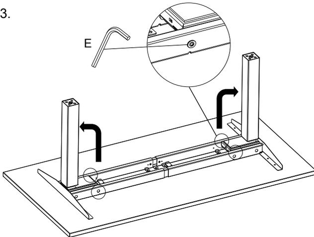
Set the column straight, then tighten the screws inside the main frame
