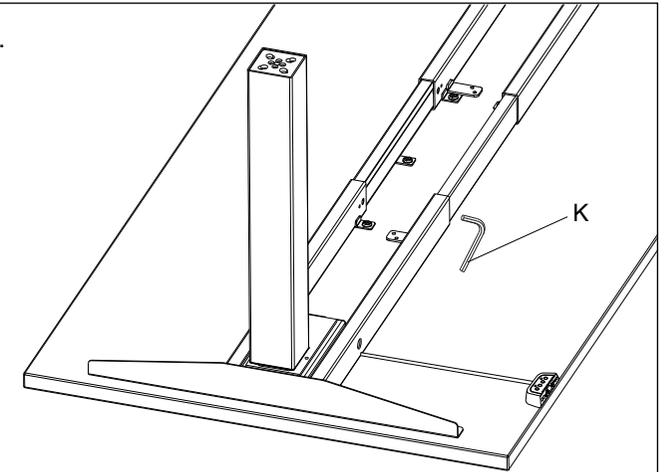
Tighten up the pre-installed screw
